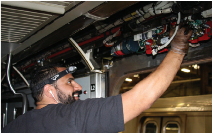
CIB Nelson Matos installs door controller.
