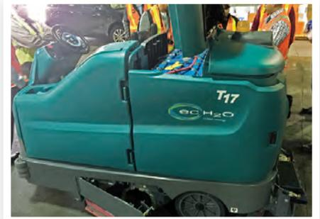
**The MTA is beginning to replace diesel powered scrubbers and sweepers with battery powered equipment.**
